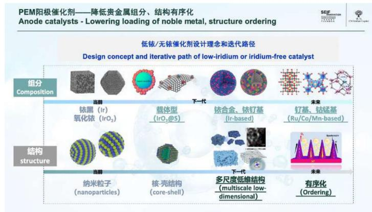
**Slide 10 appears to explore the design and development of anode catalysts for PEM electrolyzers with an emphasis on reducing the use of expensive noble metals like iridium and enhancing the structure ordering of the catalysts.**
