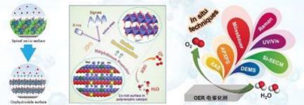
• Ir、Ru基析氧催化剂在高电位下易发生表面重构 (Surface reconstruction)
