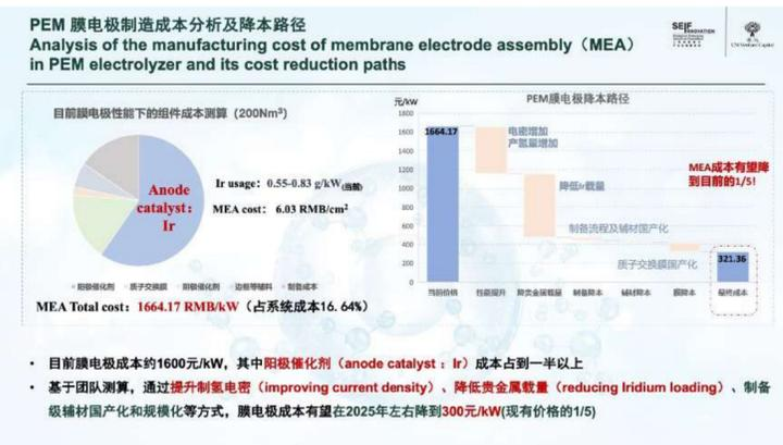
**Slide 5 presents an analysis of the manufacturing cost of Membrane Electrode Assembly (MEA) in PEM electrolyzers and discusses potential pathways for cost reduction.**
