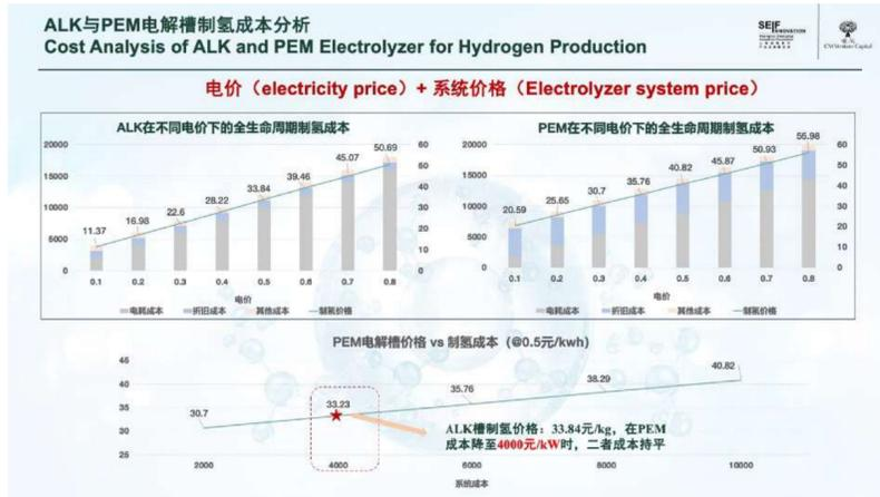
Slide 3 is titled "Cost Analysis of ALK and PEM Electrolyzer for Hydrogen Production," which compares the costs associated with Alkaline (ALK) and Proton Exchange Membrane (PEM) electrolyzers used in hydrogen production.
